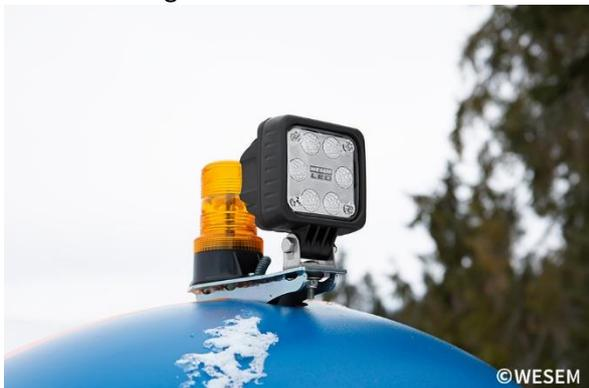
Still, customers' expectations are also well met by CRC3 work lamps, which have excellent technical characteristics and feature an option to choose various lamp shapes. The lamps are easy to mount or to replace, and do their job perfectly.
